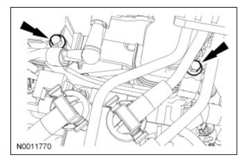
17. Connect the ignition coil electrical connector.
