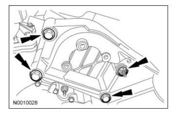
24. Position the power steering pump and install the 3 bolts.Tighten to 25 Nm (18 lb-ft).
