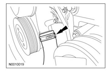
35. Connect the upper radiator hose to the thermostat housing.
