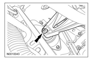
3. Install the LH engine mount nut.Tighten to 63 Nm (46 lb-ft).
