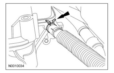
14. Attach the crankcase vent tube to the LH valve cover.
