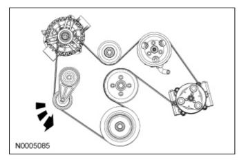
27. Tighten the 3 power steering pulley bolts.Tighten to 25 Nm (18 lb-ft).
