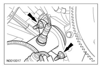
40. Connect the 2 Heated Oxygen Sensor (HO2S) and the 2 Catalyst Monitor Sensor (CMS) electrical connectors (1 shown).
