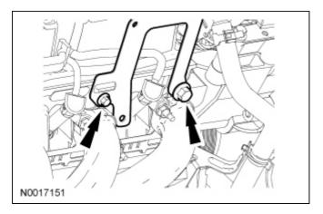
22. Connect the 2 heater hoses to the coolant tube.
