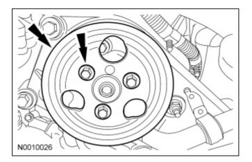
26. Rotate the accessory drive belt tensioner counterclockwise and install the accessory drive belt.
