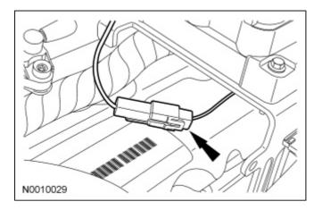
19. Attach the spark plug wire retainer to the intake manifold.
