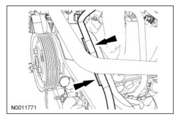
30. Connect the A/C compressor and A/C high pressure switch electrical connectors.
