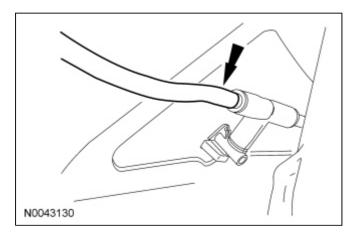
43. Install the 1 hood insulation pin-type retainer and attach the 2 windshield washer hose retainers.
