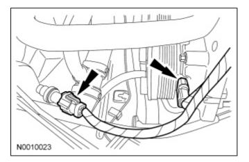
31. Connect the Power Steering Pressure (PSP) switch electrical connector.
