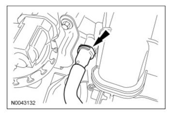
13. Connect the brake booster vacuum hose to the upper intake manifold.
