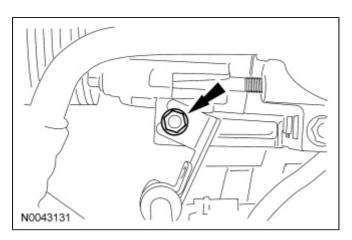
34. Connect the lower radiator hose to the coolant pump.
