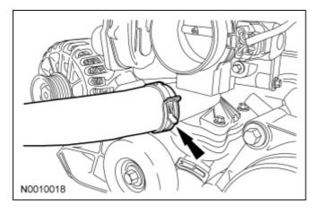
36. Position the ground strap and install the stud bolt.Tighten to 10 Nm (89 lb-in).
