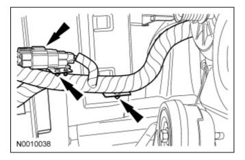
11. Connect the upper and lower PCM electrical connectors.
