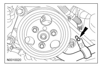
33. Position the Power Steering Pressure (PSP) tube bracket on the A/C compressor and install the nut.
