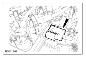
18. Connect the radio ignition interference capacitor electrical connector.
