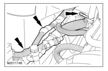
10. Connect the 16-pin electrical connector and attach the 2 wiring retainers.
